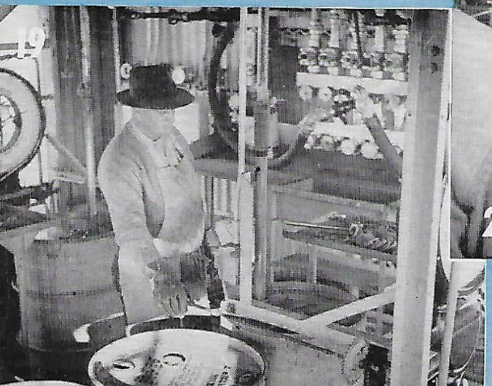
(19) At a "light products" filling station George Neil compensates for varying barrel weights by always adjusting scale to "0", which then automatically "weighs in" 53 gallons. (20) Full drums move to warehouses by roller conveyor and are sorted into commodity classifications by push-button. (21) Finally, Frank Mathos, lifting four barrels at once, climaxes our tour of Barrel Utopia.
