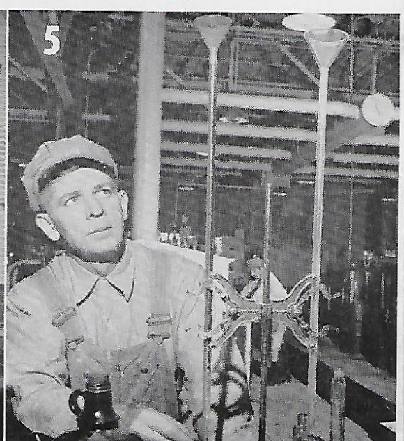
(4) This "decontaminator," employing jets of hot air and steam, eliminates explosive vapors, dislodges dirt and oil, and removes contaminants by vacuum. (5) Julius Wennerholm depends upon laboratory methods and equipment to test the cleansing potency of a caustic soda solution next used in the elaborate cleaning process. . . .
