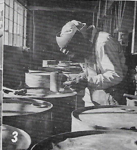
(1) Here we are in Oleum Refinery's "raw drum" storage area where thousands of used company barrels have returned from all points of the compass for re-use. (2) John Souza, with drum under press and full of water, will use 80 pounds of water-pressure to remove dents. (3) Seen welding a damaged bung is Joseph Horvat. . . .
